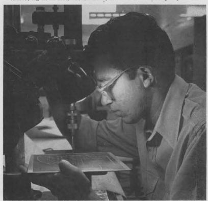
PRECISION DRILLING with a tolerance of .005-in. is done optically by George Hernandez. The holes in the printed circuit card are for eyelets or they are plated to allow flow-through of current from one side of the card to the other to continue circuit.
